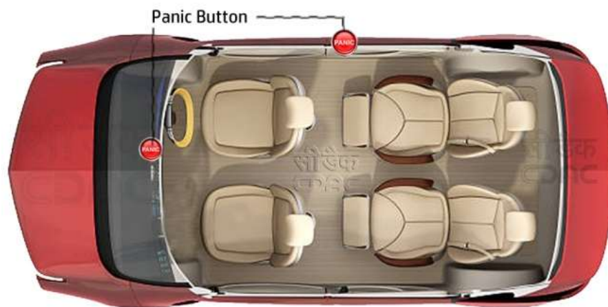
Figure3: Indicative Panic Button positions for car
